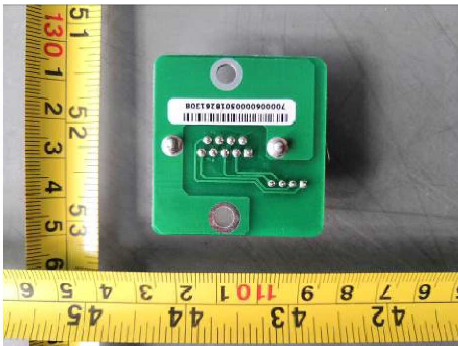
RS232 board solder side view
