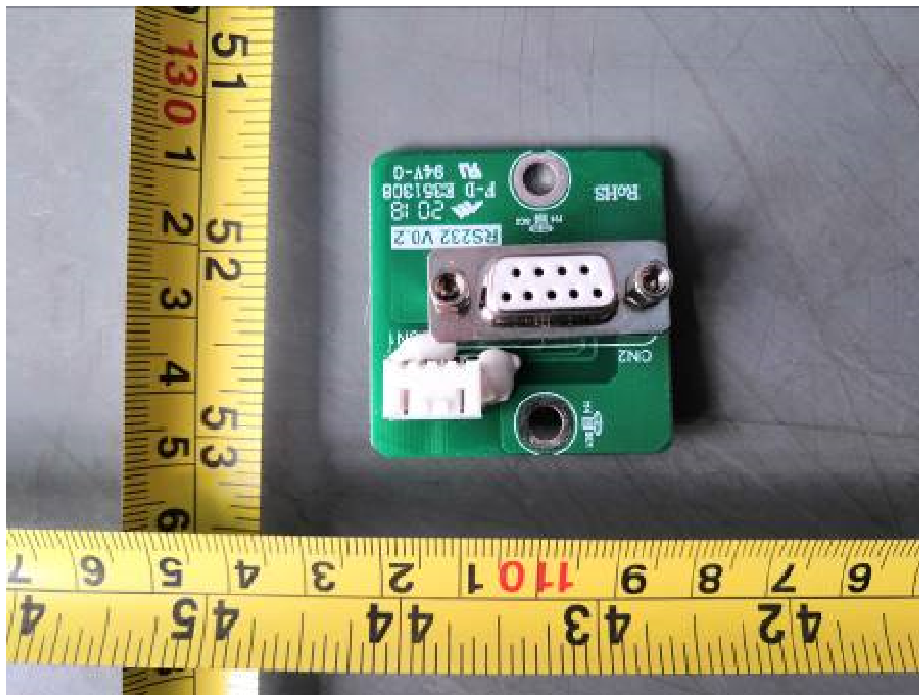
RS232 board solder side view
